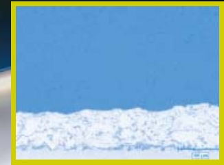
Cr 2 O 3 – porosity < 1 % hardness 1500 - 1550 Hv
